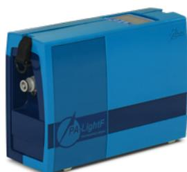
**Light-915** is a compact light-weight instrument for workplace monitoring, pollution revealing and mapping, and mercury spill clean-up verification. As compared to RA-915M, it is equipped with a shorter analytical cell to expand the measurement range up to mg/m<sup>3</sup> and simpler interface and is intended for measuring higher mercury concentrations. Data logger has capacity for 122 hrs data acquisition.
