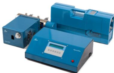
**PYRO-915+ attachment** implements unique advantages of Zeeman AAS: direct analysis of any solid and liquid samples excluding sample preparation procedures. The PC programmable heating modes and full control over atomization process makes it possible to optimize analysis conditions for specific samples over a wide range of the mercury concentrations.
